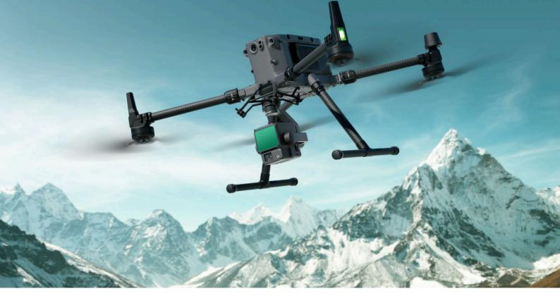
Zenmuse L2 is a high-precision aerial LiDAR system that empowers drones with more accurate and efficient 3D data collection. With 4cm vertical accuracy, 5cm horizontal accuracy, and the ability to cover an area of 2.5 km<sup>2</sup> during a single flight, this IP54-rated system allows users to effortlessly handle a wide range of operational scenarios.
