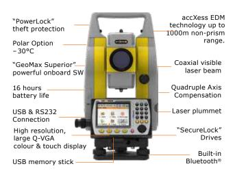
With the proven accXess technology, the Zoom50 features intelligent distance measurement engine designed for outstanding range, speed and highest accuracy even under tough conditions. The longer measurement range means a wider operational coverage and significant less time lost with switching setups. The new "PowerLock" protection mechanism prevents the use by unauthorized persons and makes it unattractive to steal.
